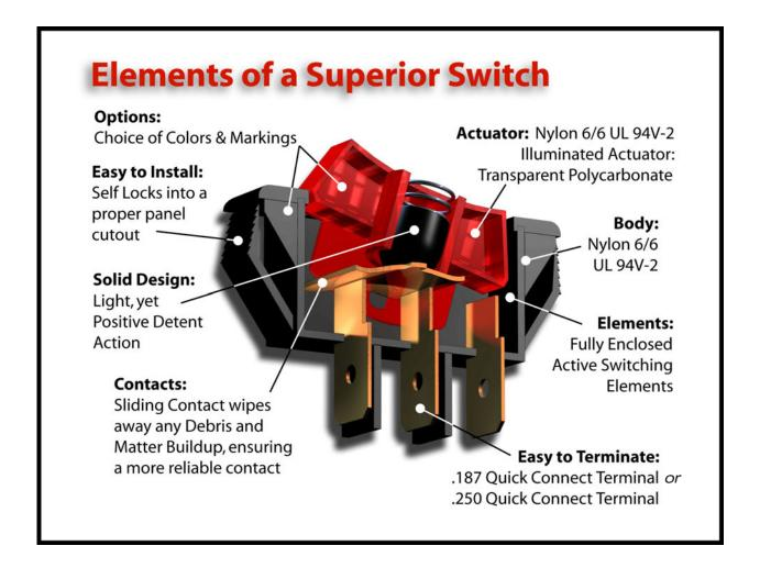
Many of Sigma Switches' switches have a self cleaning contact feature. Unlike most rocker switches, Sigma's contacts are manufactured to slide and rotate with each actuation of the switch wiping away matter buildup and maintaining contact cleanliness.
